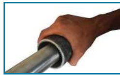
Step 3: Chamfering the Tubes
