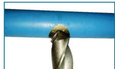
Step 3: Drilling the Required Hole on the tube
