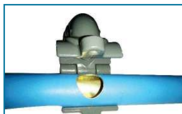
Step 5: Aligning the Droplet to the hole
