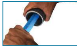
Step 3: Chamfering the Tubes
