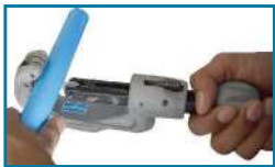
Step 1: Cutting the Tubes
