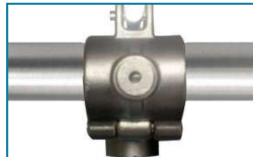
Step 2: Marking the position of the hole on tube
