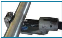
Step 1: Cutting the Tubes
