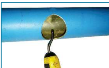
Step 4: Chamfering the hole
