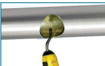
Step 4: Chamfering the hole
